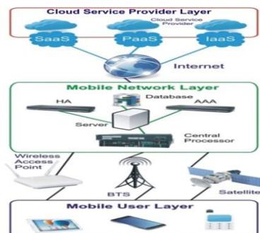
Figure 1: The architecture of Mobile Cloud Computing
